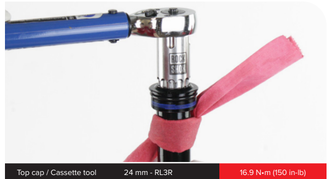
Top cap / Cassette tool 24 mm - RL3R 16.9 N·m (150 in-lb)
